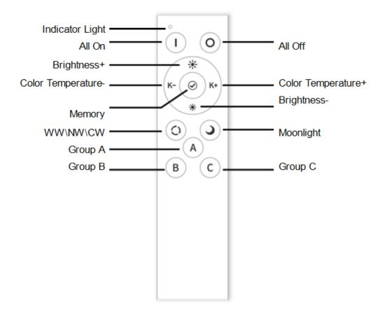
**Brightness+/-** press the button, can adjust the brightness 10%~100%
